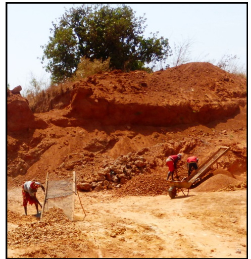
Surface workers grading laterite to make various grades of building resource
