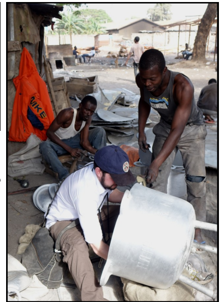
Guy gets down to work, helping the aluminium recyclers finish a large cooking pot after it has been taken from the mould and allowed to cool
